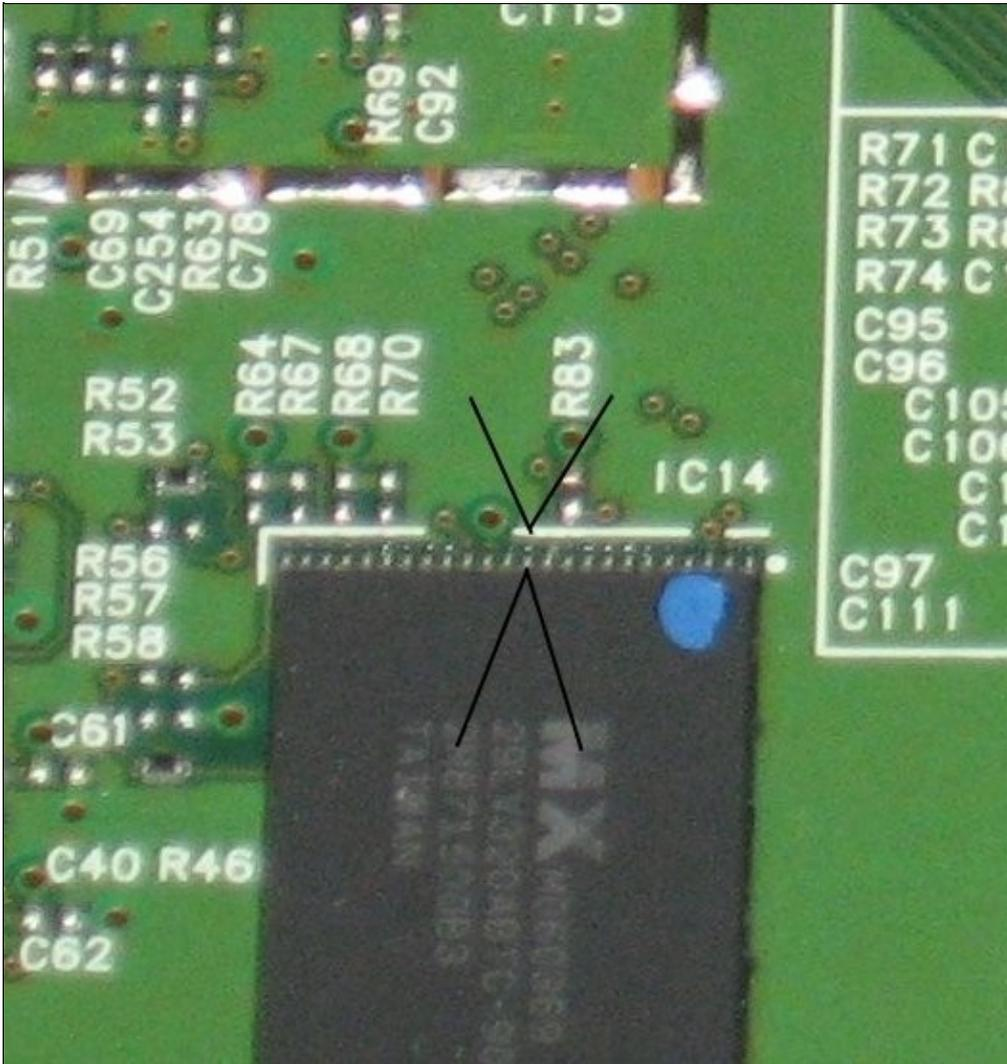
..... It is the 12th pin counter-clockwise from the dimple in the surface of the chip. See the specs for this chip [here](#). This is the Reset pin.
